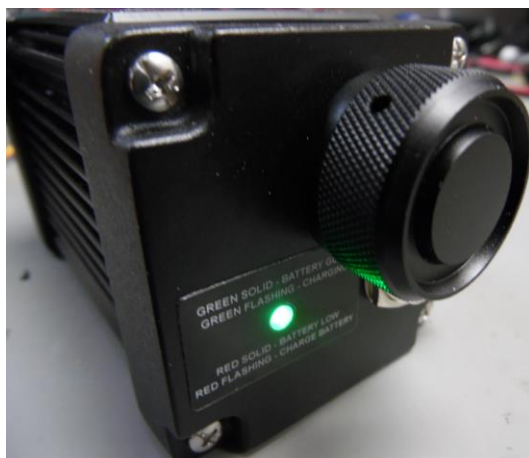
Figure 5: Rotary switch and power LED.
