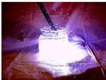
Figure 2: Igniter firing in water.
