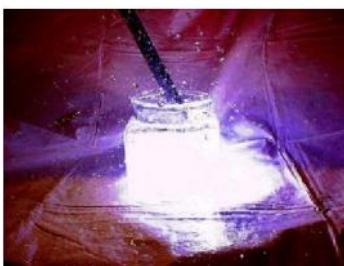
Figure 2: Igniter firing in water.
