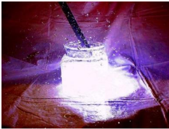
Figure 2: Igniter firing in water.
