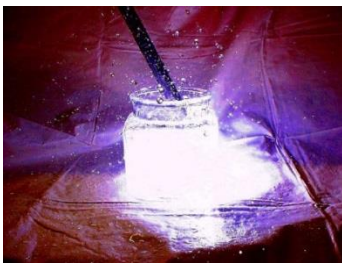
Figure 2: Igniter firing in water.
