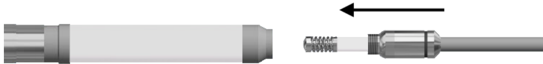
Figure 5: Igniter installation into Triaxial Rod.
