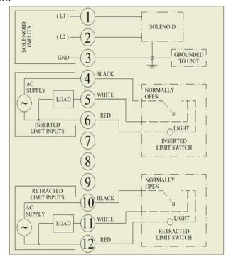
Figure 5: System Schematic Diagram with 2 limit switches
