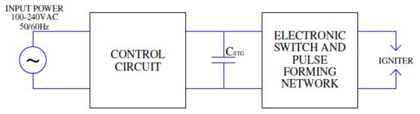
Figure 1: High Energy Exciter basic schematic.
